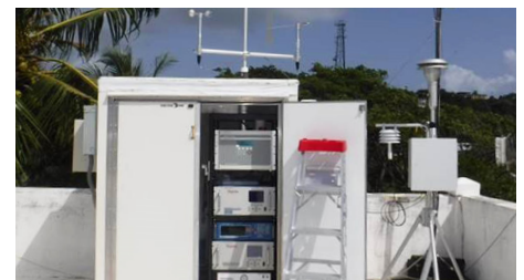
Former Vieques Naval Training Range, Monitoring for PM10, CO, Metals and Explosives
